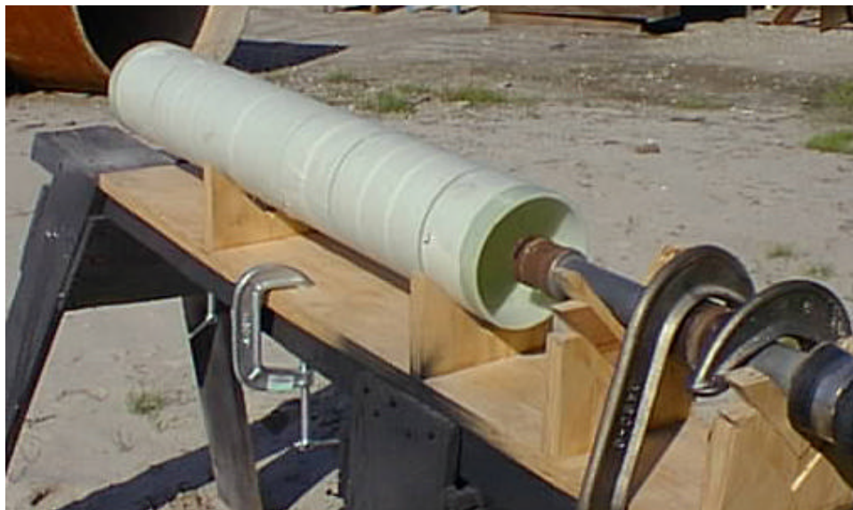
FIGURE 1 - Test setup for sandblasting assembled pipe specimen.
