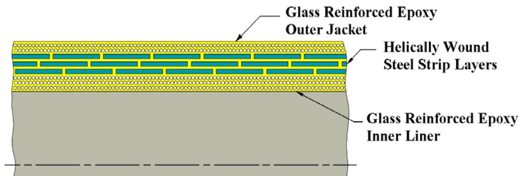
Figure 1. Wall Construction of SSL Pipe.
